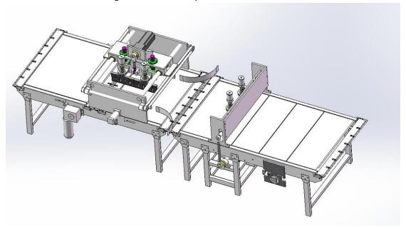
The width of the tape along which the product will move 1000mm, the speed of the product will be regulated from 1m / min to 2m / min, the product is cut to 60mm.
